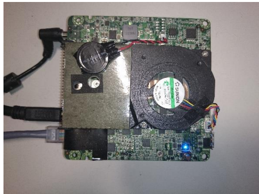
Fig. 7. 4"x4" NED prototype (~10.1x10.1 cm 2 )
